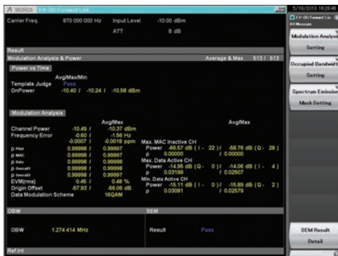
All Measure Screen: EV-DO Forward Link
