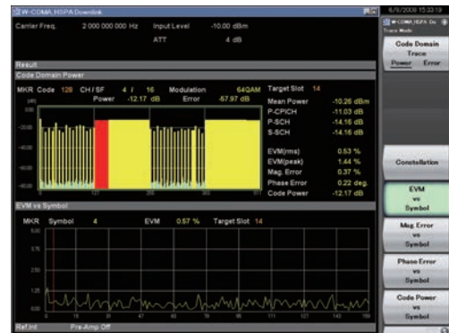
Code Domain (Vector Error vs. Symbol)
