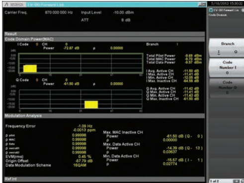
Code Domain Power Screen: EV-DO Forward Link
