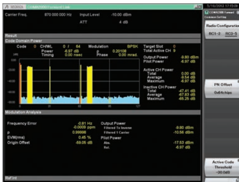
Code Domain Screen: CDMA2000 Forward Link
