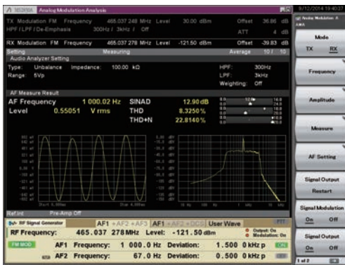
Example of RF Signal Output and AF Signal Measurement Screen (with Analog Signal Generator and Audio Analyzer Options)
